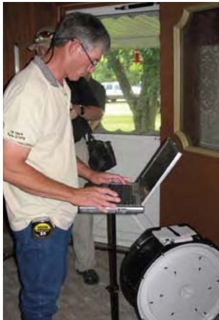
This photo depicts a blower door test, which is used to analyze a home’s energy efficiency.
